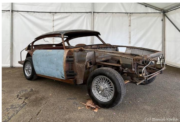
Aston Martin DB6 with tubular framework.
